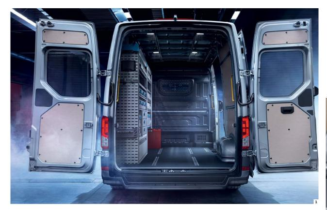
**01 Rear wing doors\*.** The two roof-height doors provide an opening angle of 180°.
