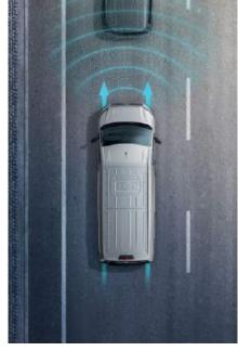
Front Assist with City Emergency Braking System.
