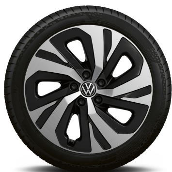
STANDARD ON ID.4 City 18" 'Falun' alloy wheels 8J x 18 in front, 9J x 18 in rear Tyres: 235/50 R18 in front 255/45 R18 in rear
