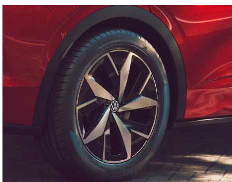
STANDARD ON ID.4 GTX 20" 'Ystad' alloy wheels 8J x 20 in front, 9J x 20 in rear Tyres: 235/50 R20 in front 255/45 R20 in rear
